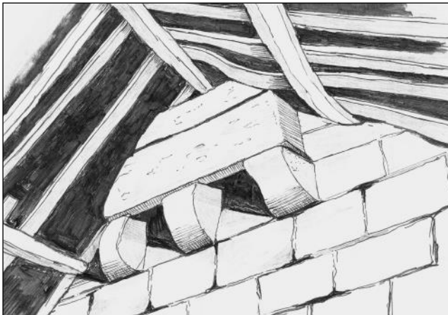
Jackson's Farm, Worsthorne – drawn September 2015. Internal corbelled cap for firehood.
